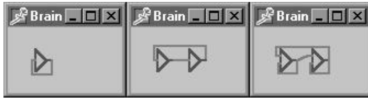
Figure 4. Figures 4a, 4b, and 4c depict three central pattern generator networks of increasing complexity. They are, respectively, a single neuron with a single connection, two neurons with two connections, and two neurons with four connections.
