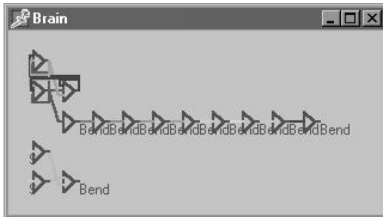
Figure 10. The nervous system of the 2-D food finder depicted in figure 9. A central pattern generator drives a chain of muscles in the creature's tail. A pair of sensors and a single left-right steering muscle constitute the creature's stimulus orientation network.
